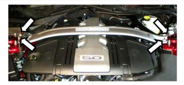
Remove the stock engine cover. Using a small flat blade screw driver, carefully remove the (2) round covers located at the front right & left of the engine cover. Using a 10mm socket, remove the retaining nuts from both locations. Remove the cover and set aside, with the nuts, in a safe location for reinstallation.
