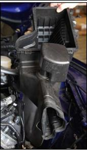
7. Install the PMAS heat shield in the stock air cleaner housing location. Align the upper mount tab with the stock mount location and install the stock mount bolt retained from housing removal, **DO NOT TIGHTEN**. Push the rubber Wellnut into the hole in the inner fender well. Once it's fully seated against the fender well, use a 3/16" allen wrench to tighten the socket head screw securely. Using a 10mm socket, tighten the stock mount bolt.
