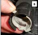
Loosen the hose clamp at throttle body inlet and release the retainer clips for the air cleaner lid. Remove the intake tube/air cleaner lid assembly from the engine bay and set aside.
